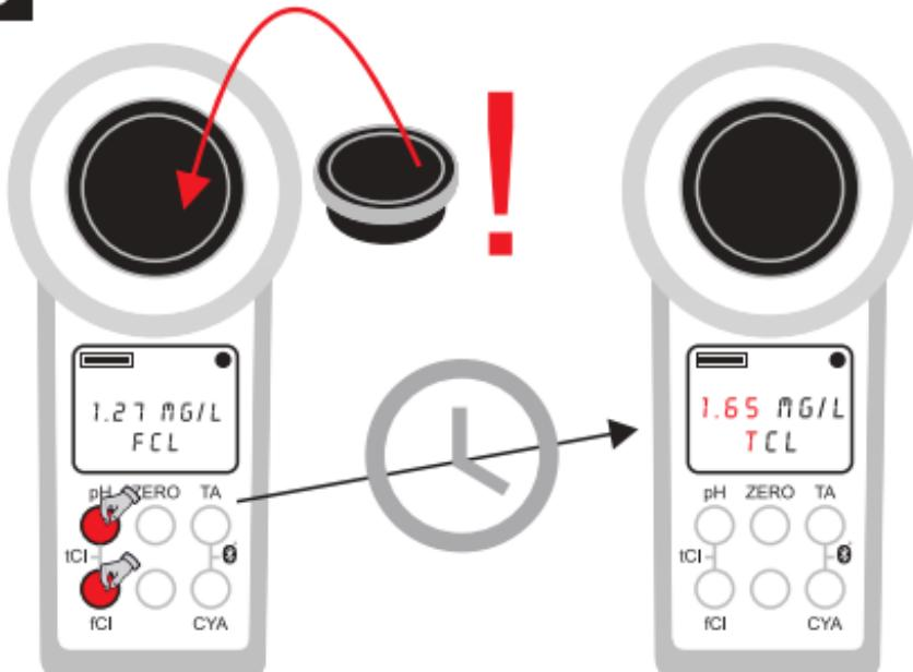
Total Chlorine is measured directly after free Chlorine without emptying the cuvette. The DPD 3 tablet is added to the sample water which already contains the DPD 1 tablet (dissolved). Combined Chlorine is calculated as Total Chlorine minus free Chlorine.
